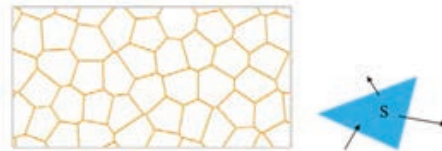
Fig. 6.1. Arbitrary unstructured grid on the left. A schematic illustration of the finite-volume numerical procedure on the right.
