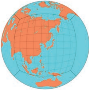
Fig. 2.1. Example of Cubed-sphere grid system used in KIM
