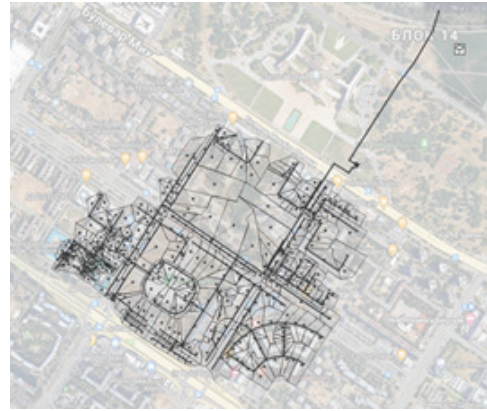
Fig 1. Schematic of the Block 13 case study drainage network. (Source: author no. 1, based on the supplied Block 13 SWMM model provided by the FCE-UB.)
