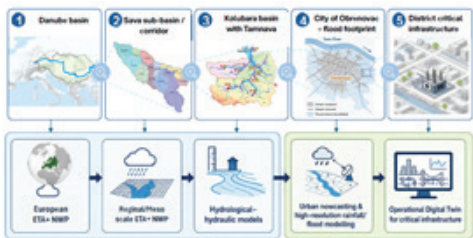
Figure 2: Multiscale spatial and modelling nesting from the Danube-Sava-Kolubara-Tamnava basin to the Obrenovac flood footprint and district critical infrastructure within the Local Digital Twin framework
